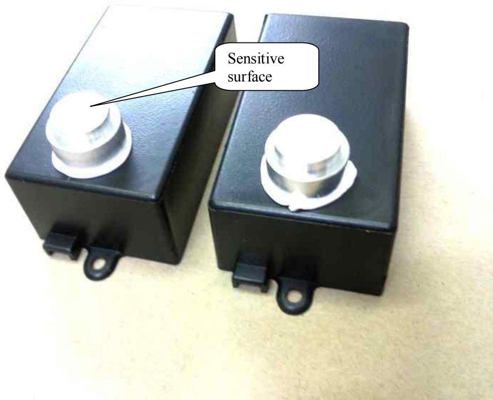
Figure 2 eTarget sensors HEXU-0000 with built-in active filters, analogue signal pre-processor
